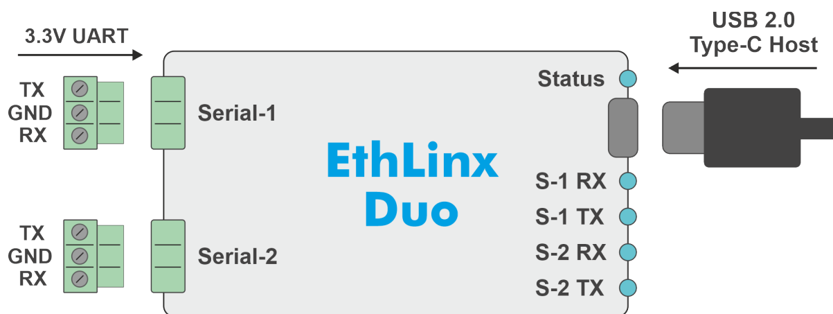
Image 2: Basic Wiring Diagram with serial connections and LED description – EthLinx Duo
