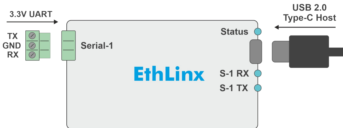
Image 1: Basic Wiring Diagram with serial connections and LED description - EthLinx
